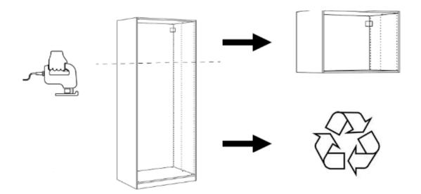
**Step 02:** Once the PAX is cut, we will turn it upside down, making the top cover the base of the top cabinet. In this way, the cut of the wardrobe will be on the top area, and the joining of both shells will be cleaner and more precise.
