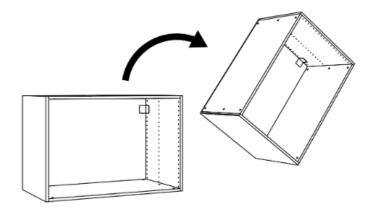
**Step 03:** The top cabinets are screwed from the "new base" to the lower PAX and also between them, to achieve a completely compact and solid structure.
